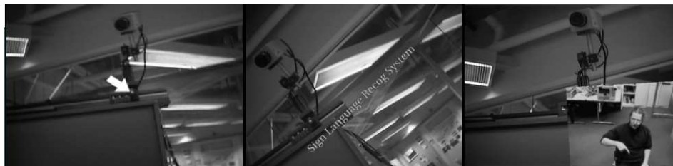
Figure 2: When a tag is first located, a red arrow is used to indicate a hyperlink. If the user shows interest by staring at the object, the appropriate text labels are displayed. If the user approaches the object, 3D graphics or movie sequences are shown.
