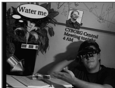
Figure 1: Multiple graphical overlays aligned through visual tag tracking. Such techniques as shown in the following 3 images can provide a dynamic, physically-realized extension to the World Wide Web.
