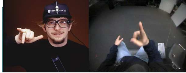
Figure 6: The baseball cap mounted camera and its perspective.
