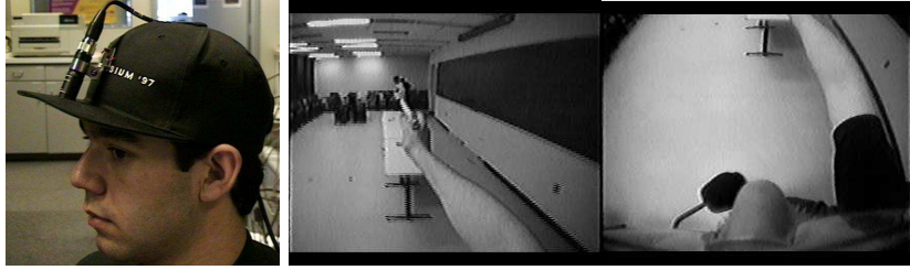
Figure 7: Left: The two camera Patrol hat. Right: the downward- and forward-looking Patrol views.
